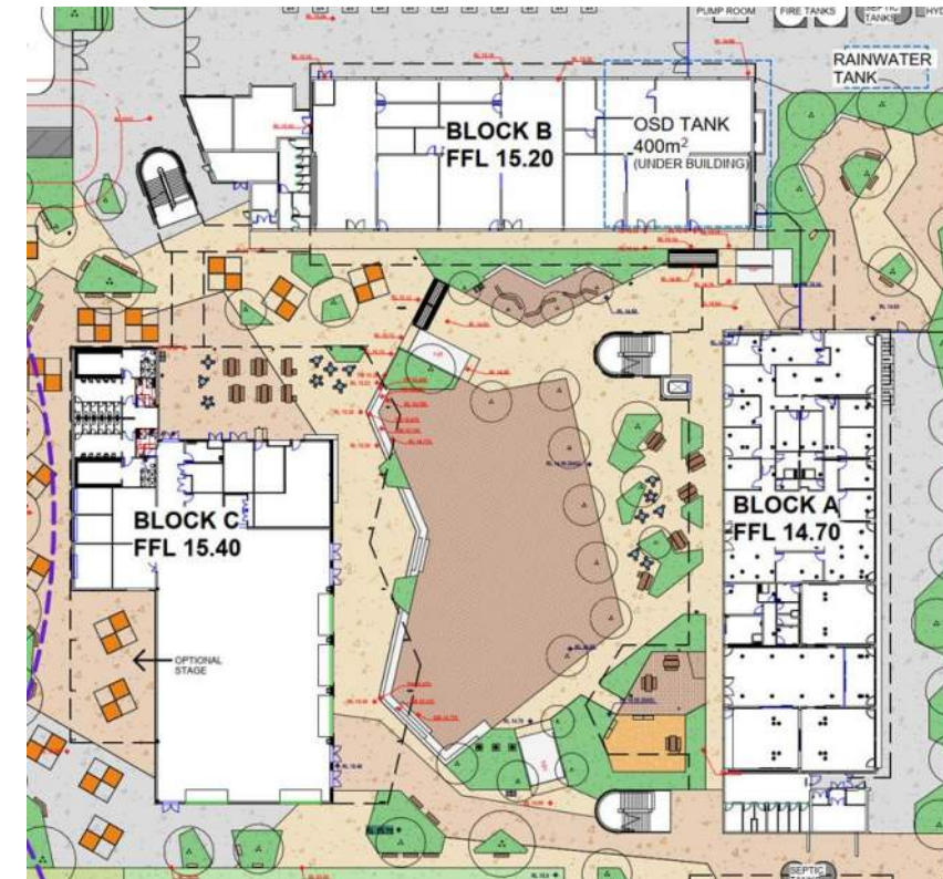
Figure 6 Flood Planning Levels (background by NBR)
